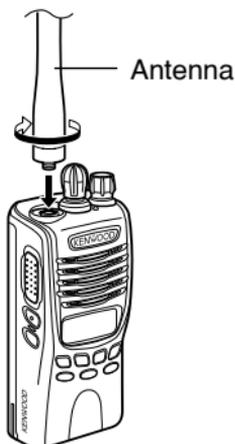
Screw the antenna into the connector on the top of the transceiver by holding the antenna at its base and turning it clockwise until secure.
