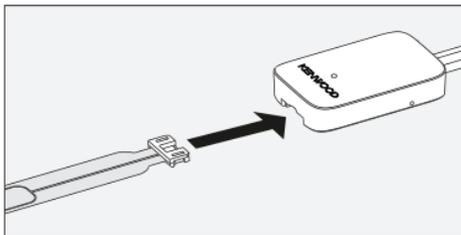
6. Insert the DAB film aerial into the slot in the antenna.
