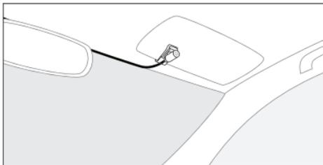
1. If possible, tuck the cable into the roof lining, keeping the microphone near the driver's position. Alternatively, use self-adhesive clips to fix the microphone cable along the top of your windscreen.
