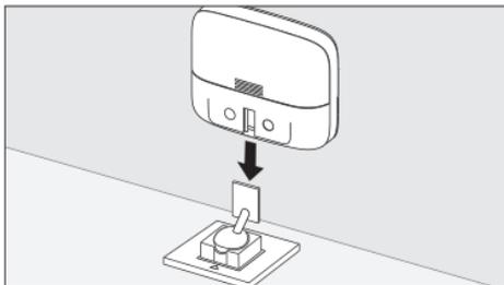
3. Peel off the backing from the wireless controller bracket and gently stick it onto your dashboard. Gently press the bracket to ensure it's attached securely.
