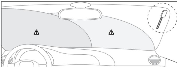
If you have a heated windscreen in your vehicle, or the windscreen contains metallic UV filters, it can cause interference for the DAB signal. Install the antenna on a part of the windscreen that does not contain heating elements or UV filters.
