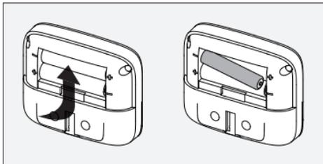
1. Slide the back cover off of the wireless controller and insert the batteries, then replace the cover.
