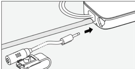
1. Insert the microphone connector into the socket at the top of the antenna, until it clicks into place.
