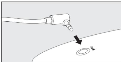
5. If you're connecting your KTC-500DAB with an auxiliary cable, insert the cable into your vehicle's auxiliary socket. If you're connecting your KTC-500DAB by FM radio, you can store the auxiliary cable so it's out of the way.
