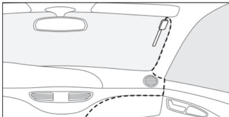
1. Place the antenna cable so that it follows a path to your vehicle's power socket.
