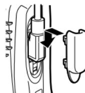
**3** While holding the locking bracket in place, push it towards the bottom of the transceiver until the tabs on the bracket click into place.
