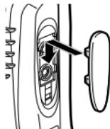
**2** While holding the cap in place, push it towards the bottom of the transceiver until the tabs on the cap click into place.
