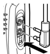
**2** Place the locking bracket over the speaker/ microphone plugs so that the locking tabs insert into the transceiver grooves.
