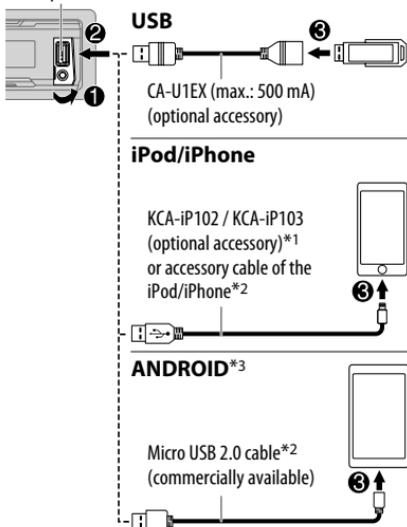
\*1 KCA-iP102 : 30-pin type, KCA-iP103 : Lightning type
