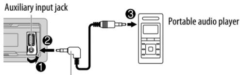
3.5 mm stereo mini plug with "L" shaped connector (commercially available)
