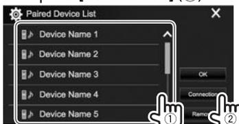
4 Select [ON] (to connect) or [OFF] (to disconnect) for the target (①), then display the <Paired Device List> screen (②).
