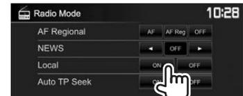
The unit tunes in only to stations with sufficient signal strength. The LO.S indicator lights up.
