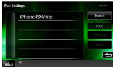
If a connectable Bluetooth device is not displayed, touch [Search] and do the pairing of the devices.
