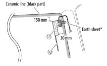
\* Attach the earth sheet of the amplifier unit (①) to the metal part of the front pillar.
