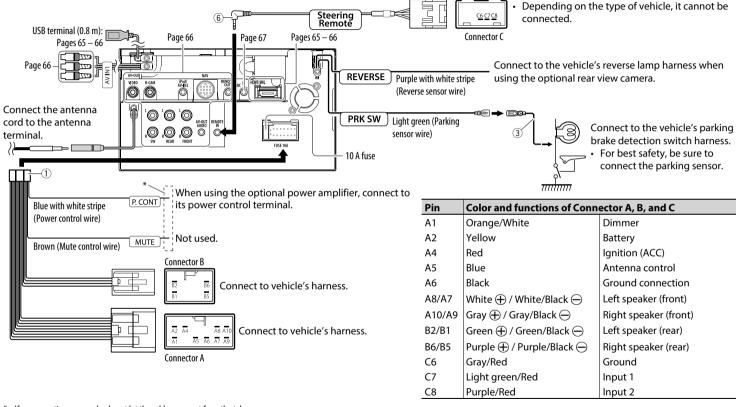
Connect to the vehicle's steering remote harness.
