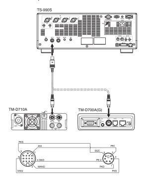
Be sure that "On" has been configured for both Advanced Menus 14, "PKS Polarity Reverse", and 15, "TX Inhibit While Busy". Refer to "INHIBITING THE TRANSMISSION DURING BUSY (SQUELCH OPENING)" and "REVERSING THE PKS SIGNAL POLARITY" for the configuration methods.
