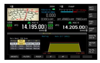
3 Press [FILTER] (F2) or [FIL/SEL] (M) to select the receive filter.
