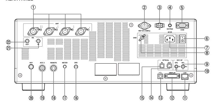
① ANT 1 to ANT 4 (Antenna 1 to Antenna 4) connectors For use with  $50\Omega$  antenna. These SO-239 / M-type coaxial connectors can connect a maximum of four antennas. {page 4-22}
