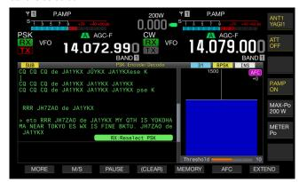
♦ If the transceiver is in any mode other than PSK mode, "TX: Reselect PSK" appears in the RTTY Encode/Decode screen. Press [FSK/PSK/REV].
