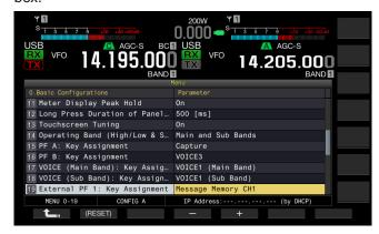
4 Press [-] (F4) or [+] (F5), or rotate the MULTI/CH control to select the function to be assigned to a PF kev.
