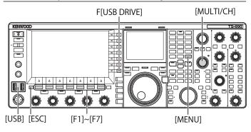
Insert a USB flash drive to the (USB-A) connector.
