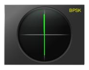
Tuned Correctly (BPSK Mode)
