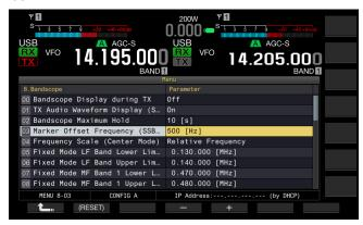
4 Press [-] (F4) or [+] (F5) to select "Off (Carrier Point)" or the offset frequency.
