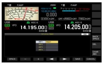
4 Enter the antenna name by pressing the function keys or rotating the MULTI/CH control.
