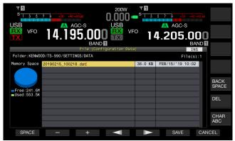
5 Use the functions keys and the MULTI/CH control to edit or enter a text string for the file name.
