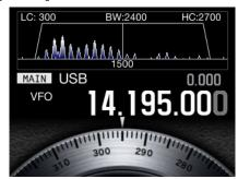
The Sub Scope with Waveform displayed
