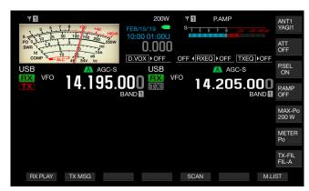
In the key guide [P.SEL] (F), the status of attenuator is indicated on the lower line.
