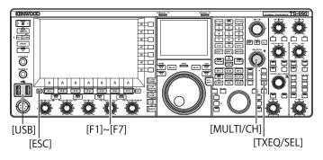
1 Press and hold [TXEQ/SEL] to open the TX Equalizer screen.
