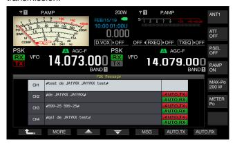
You can configure the transceiver so that the transceiver will revert to a receive state after an PSK message is transmitted from the corresponding channel when "AUTO RX" appears on the right side of the PSK message. Even if "AUTO RX" disappears, the transceiver does not revert to the receive mode after the PSK message for that channel is sent.
