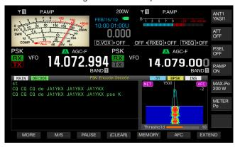
If [AFC] (F5) is unavailable in the function key guide, press [MORE] (F1). An alternate key guide will appear.
