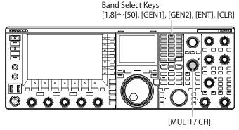
Press the band keys [1.8] to [50], [GEN1], and [GEN2] to store the frequency and operating mode.
