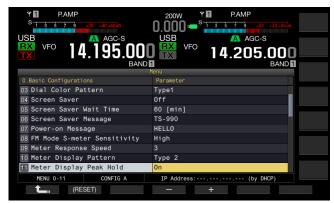
4 Press [-] (F4) or [+] (F5) to select "Off" or "On". The default is "On" (use with Meter Peak Hold). Selecting "Off" disables the Meter Peak Hold. In this case, the peak values remain displayed for the duration below.
