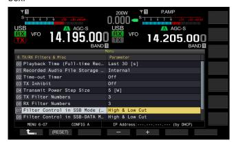
4 Press [-] (F4) or [+] (F5) to select either "High & Low Cut" or "Shift & Width" for the behavior of the control. The changes of the shift and filter type appear on the RX Filter screen. The default is "High & Low Cut".
