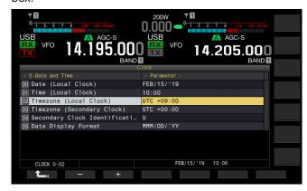
6 Press [-] (F2), [+] (F3), or rotate the **MULTI/CH** control to select the timezone for Local Clock.
