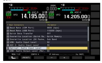
4 Press [-] (F4) or [+] (F5), or rotate MULTI/CH control to select the input level from the available range between "0" and "100".
