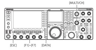
1 Press and hold [DATA/SEL] to open the Modulation Source screen.
