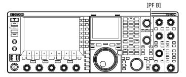
1 Press the key to which [PF B] or Voice 3 is assigned. The value of the meter when the key was pressed is announced.
