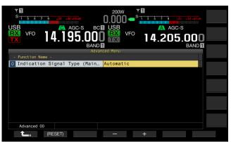
4 Press [-] (F4) or [+] (F5), or rotate the MULTI/CH control to select the signal format.
