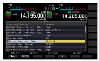
4 Press [-] (F4) or [+] (F5), or rotate the MULTI/CH control to configure the wait time until the screen saver will be activated.
