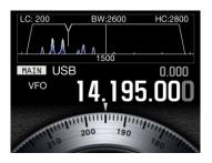
2 Rotate the **NOTCH** (M) or **NOTCH** (S) control to adjust the notch filter frequency.
