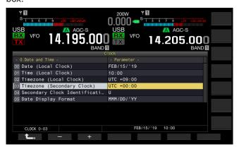
6 Press [-] (F2) or [+] (F3), or rotate the MULTI/CH control to select the timezone for the secondary clock from the available range of "-14:00" to "+00:00" to "+14:00".
