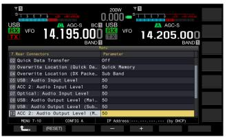
4 Press [-] (F4) and [+] (F5), or rotate the MULTI/CH control to select the audio signal output level for the main band from the available range between "0" and "100".
