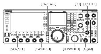
1 Receive a standard wave signal on the main band. To receive the 10 MHz standard wave signal, rotate the Tuning control to select exactly "10.000.00".
