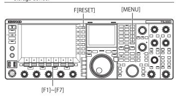
Follow the procedure below to fully reset the transceiver.
