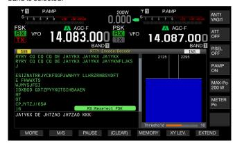
♦ If the transceiver is in any mode other than RTTY (FSK) mode, "TX: Reselect FSK" appears in the RTTY Encode/Decode screen. Press [FSK/PSK/REV].
