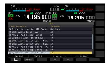
4 Press [-] (F4) and [+] (F5), or rotate the MULTI/CH control to select the audio signal output level for the main band from the available range between "0" and "100".
