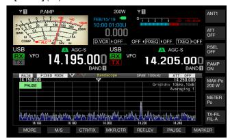
Pressing any key other than [MORE] (F1) and [MARKER] (F7) releases the pause of the waveform display.
