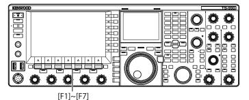
1 Press [RF/AF] (F1) on the Bandscope screen to open the Audio Scope screen.
