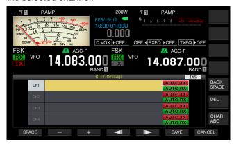
6 Use functions keys, the MULTI/CH control, or a USB keyboard to enter a text string.
