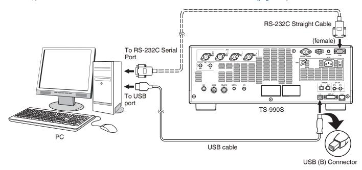
Configure the transceiver as follows according to the method of connection with the PC, the specification of the software used for data communication and the settings, etc.
