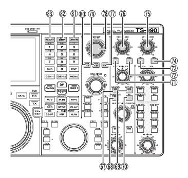
(M) Notch Filter (Main band) key: [NCH/SEL] (M) Press to toggle the Manual Notch Filter for the main band between active and inactive. {page 6-10}
