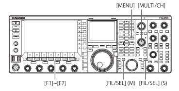
Press [FIL/SEL] (M) or [FIL/SEL] (S) to switch the receive filter.
