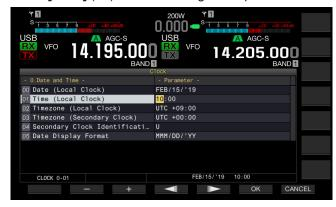
6 Use the numeric and band select keypad, function keys and the **MULTI/CH** control to configure the time. [-] (F2), [+] (F3), **MULTI/CH** control: Displays the previous parameter or the next parameter.
