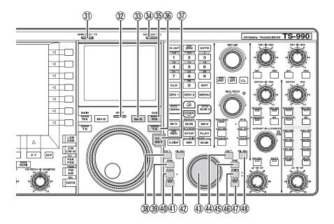
TX (Main band) key: [TX] (M) Press to switch Split mode to Simplex mode. {page 5-1}
