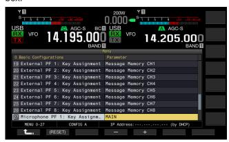
4 Press [-] (F4) or [+] (F5), or rotate the MULTI/CH control to select the function to be assigned to a PF key.
