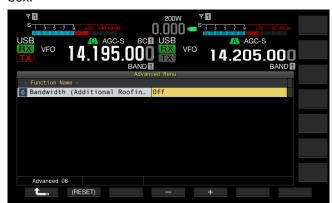
4 Press [-] (F4) or [+] (F5), or rotate the MULTI/CH control to select the passband width.
