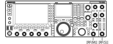
1 Rotate the RF (M) or RF (S) control to adjust the RF gain.
