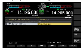
6 Use the function keys and the MULTI/CH control to enter the NTP server address.
