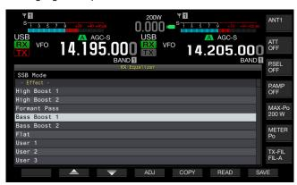
Press [ ] (F2) or [ ] (F3), or rotate the MULTI/CH control to select the desired equalizer characteristics.
