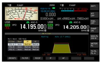
Rotate the LO/WIDTH control to change the passband width.
