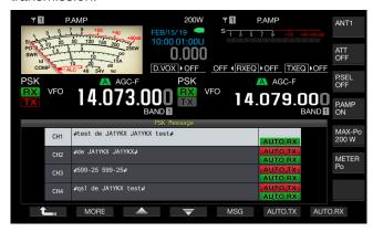
The transceiver can be configured to allow an RTTY message to be transmitted automatically from the corresponding channel when "AUTO TX" appears on the right side of the RTTY message. Even if the "AUTO TX" disappears, the PSK message for that channel is temporarily stored in the buffer for a text string and will not automatically be sent.
