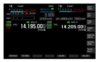
S-meter for the sub band appears on the upper right side of the main display.
