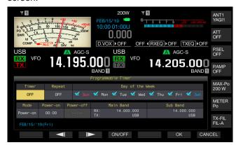
4 Use the function keys and the MULTI/CH control to configure the Programmable Timer.
