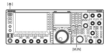
1 Hold down [M.IN] (Memory), then press [4]. After startup, the Firmware Update screen appears, and shows the firmware version.
