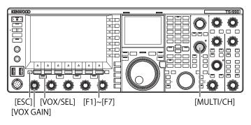
Press and hold [VOX/SEL] to open the VOX screen. In the VOX screen, a line highlights the selected audio source, and a row highlights the selected configuration item.
