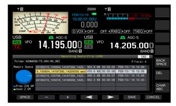
5 Use function keys, the MULTI/CH control, or a USB keyboard to enter the name.
