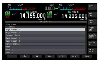
3 Press [ ] (F2) or [ ] (F3), or rotate the MULTI/CH control to select the desired characteristics.
