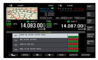
6 Press [AUTO.RX] (F7) to enable the automatic transmission.
