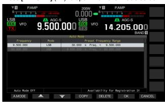
3 Press [A.MODE] (F1) to toggle the Auto Mode between active and inactive.
