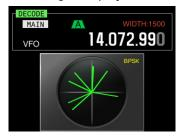
The sub-screen cycles as follows: Vector scope > Main band frequency and dial > Main band frequency and sub band frequency > Vector scope
