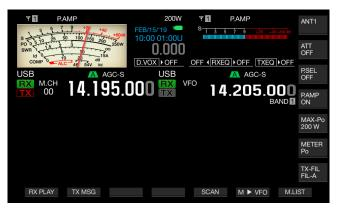
2 Press [M/V] again to exit Single-band Memory Channel mode.
