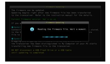
Insert the USB flash drive containing the firmware data file into the •<- (USB-A) connector on the front panel. The firmware updating progress bar appears on the main screen. Upon completion of the firmware updating, "The firmware update is completed" appears on the main screen.
