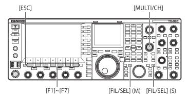
1 Press and hold [FIL/SEL] (M) or [FIL/SEL] (S) to open the RX Filter screen.
