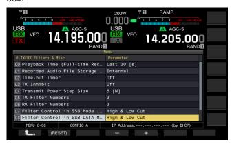
4 Press [-] (F4) or [+] (F5) to select either "High & Low Cut" or "Shift & Width" for the behavior of the control. The changes of the shift and filter type appear on the RX Filter screen. The default is "High & Low Cut".
