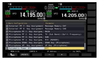
4 Press [-] (F2) or [+] (F3) to select "OFF" or the length of time until the transceiver (Φ) turns OFF.
