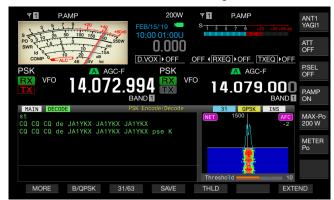
If [B/QPSK] (F5) is unavailable in the function key guide, press [MORE] (F1). An alternate key guide will appear.
