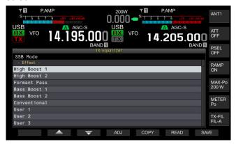
3 Press [ ] [F2] or [ ] [F3], or rotate the MULTI/CH control to select the desired characteristics of the speech processor.
