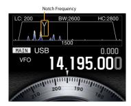
2 Rotate the NOTCH (M) or NOTCH (S) control.
