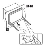
2 When the lower level is removed, remove from the upper two catches of the trim plate (5/7).
