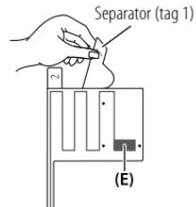
Do not touch the pasting surface (adhesive side) of the film antenna (E).
