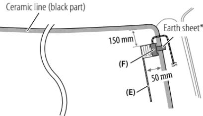
\* Paste the earth sheet of the amplifier unit (F) on the metal part of the front pillar.
