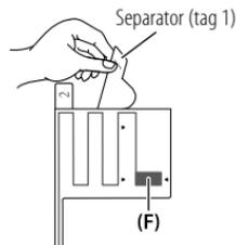
Do not touch the pasting surface (adhesive side) of the film antenna (F).
