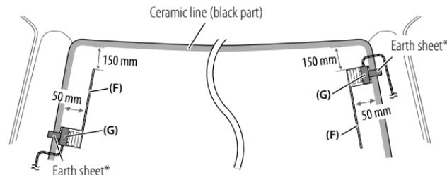
\* Paste the earth sheet of the amplifier unit (G) on the metal part of the front pillar.
