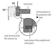
· When installing the antenna on the left side
