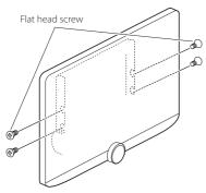
2 Adjust the display height according to the screw hole position. Default is "1".
