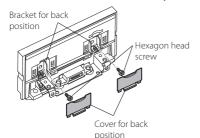
**3** Pull the slider block forward and remove the two hexagon head screws to remove the bracket for back position.
