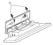
8 Attach the protective cover (accessory (2)) to coupling part, and then fix it with two binding head screws (accessory (3)).
