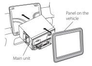
**6** Install the display unit (accessory (8)) to the main unit.
