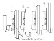
**3** Reinstall the four flat head screws on both sides and fix the display.
