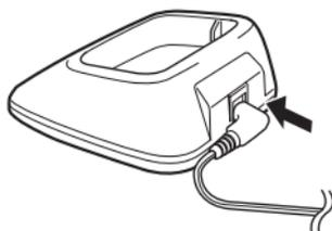
**1** Plug the AC adapter cable into the jack on the rear of the charger.
