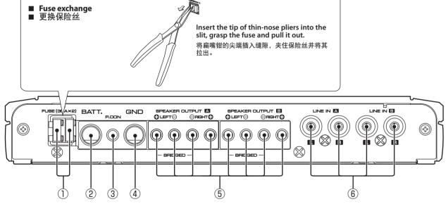
This is a 4 channel amplifier including 2 stereo amplifiers in a body. One amplifier is referred to as amplifier A and the other is amplifier B. This unit is compatible with a large variety of systems by combining the switches and functions described in the following.
