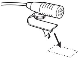
Peel the release coated paper of double-face adhesive tape to fix on the place shown above.
