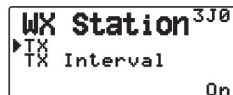
This setting determines whether or not to transmit the meteorological data obtained from the Weather Station, with the APRS data communication.
