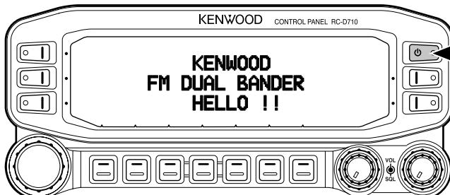
Press the [**P**] switch again to switch the transceiver OFF.
