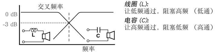
$$L = \frac{159 \times R}{f_c} \text{ (mH)} \quad C = \frac{159000}{f_c \times R} \text{ (\mu F)}$$
