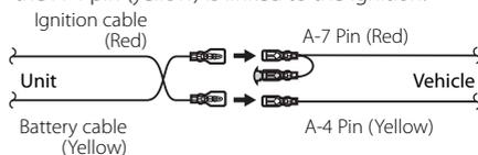
[3] The A-4 pin (yellow) of the vehicle's ISO connector is not connected to anything, while the A-7 pin (red) is connected to the constant power supply (or both the A-7 (red) and A-4 (yellow) pins are connected to the constant power supply).
