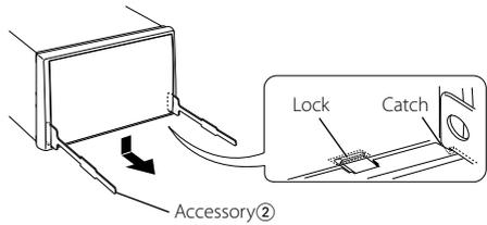
**2** When the lower level is removed, remove the upper two locations.
