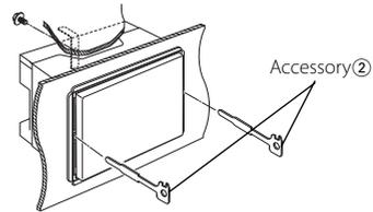
**4** Lower the removal tool towards the bottom, and pull out the unit halfway while pressing towards the inside.
