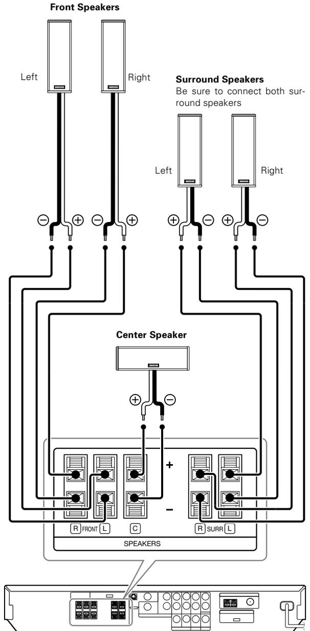
Whether each speaker is connected properly can be confirmed by outputting the test tone and checking if each speaker channel outputs audio. For details, see "Speaker settings" (Step 5 Adjust the speaker volume level). - 18
