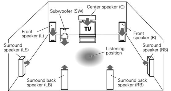
**Front speakers:** Place the left and right speakers at each side of your TV. Angle the speakers towards the listening area to enhance the stereo effect.
