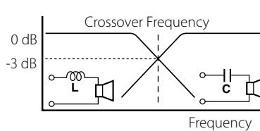
$$L = \frac{159 \times R}{f_c} \text{ (mH)} \quad C = \frac{159000}{f_c \times R} \text{ (μF)}$$
