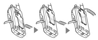
To remove the belt hook, pull the belt hook downward while pushing its tabs from both sides.
