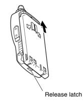
**3** To remove the battery pack, push up the release latch, then slide the battery pack back.
