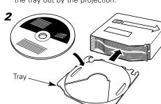
Place the disc on the tray with the label facing upwards. Insert the tray into the disc magazine until it locks. Check that the discs and trays are inserted properly. The discs are numbered from the bottom from 1 to 6
