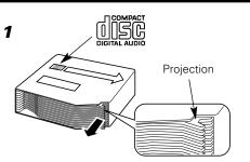
Make sure the disc magazine is the right way up with the "disc" logo on the top. Pull the tray out by the projection
