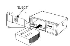
Open the CD changer door, and press the "EJECT" button.
