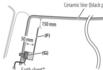
Installing the antenna on the right side
