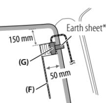
\* Paste the earth sheet of the amplifier unit (G) on the metal part of the front pillar.
