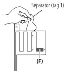
Do not touch the pasting surface (adhesive side) of the film antenna (F).
