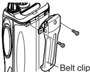
If necessary, attach the belt clip using the two supplied M3 x 8 mm screws.
