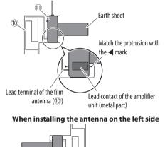
7 Remove the film covering the earth sheet and attach the earth sheet to the metal part of the vehicle.
