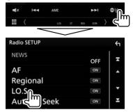
The unit tunes in only to stations with sufficient signal strength. The LO.S indicator lights up.
