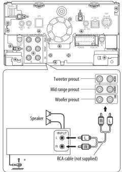
\* When connecting to an external amplifier, connect its ground wire to the car's chassis.
