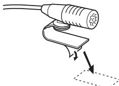
Remove the separator of the microphone, and stick the microphone to the place shown above.
