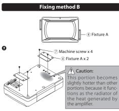
Attach the fixtures A ④ to the speaker unit securely using the machine screws ⑦. Be careful so that the connected cords do not get in between the speaker unit and fixtures A ④.
