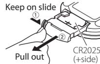
Use a commercially available button battery (CR2025). Insert the battery with the + and – poles aligned properly, following the illustration inside the case.
