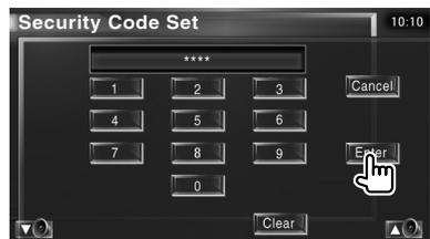
Now, your security code is registered. If you press the Reset button or if you disconnect your receiver from the battery after the code registration, you need to enter the registered security code.
