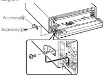
**4** Tighten the screw ( $\emptyset$ 2 × 5 mm) (Accessory **4**) and bracket (Accessory 6) in the hole shown on the diagram.
