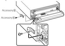
**4** Tighten the screw (Ø2 × 5 mm) (Accessory ④) and bracket (Accessory ⑥) in the hole shown on the diagram.
