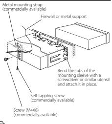
Make sure that the unit is installed securely in place. If the unit is unstable, it may malfunction (for example, the sound may skip).
